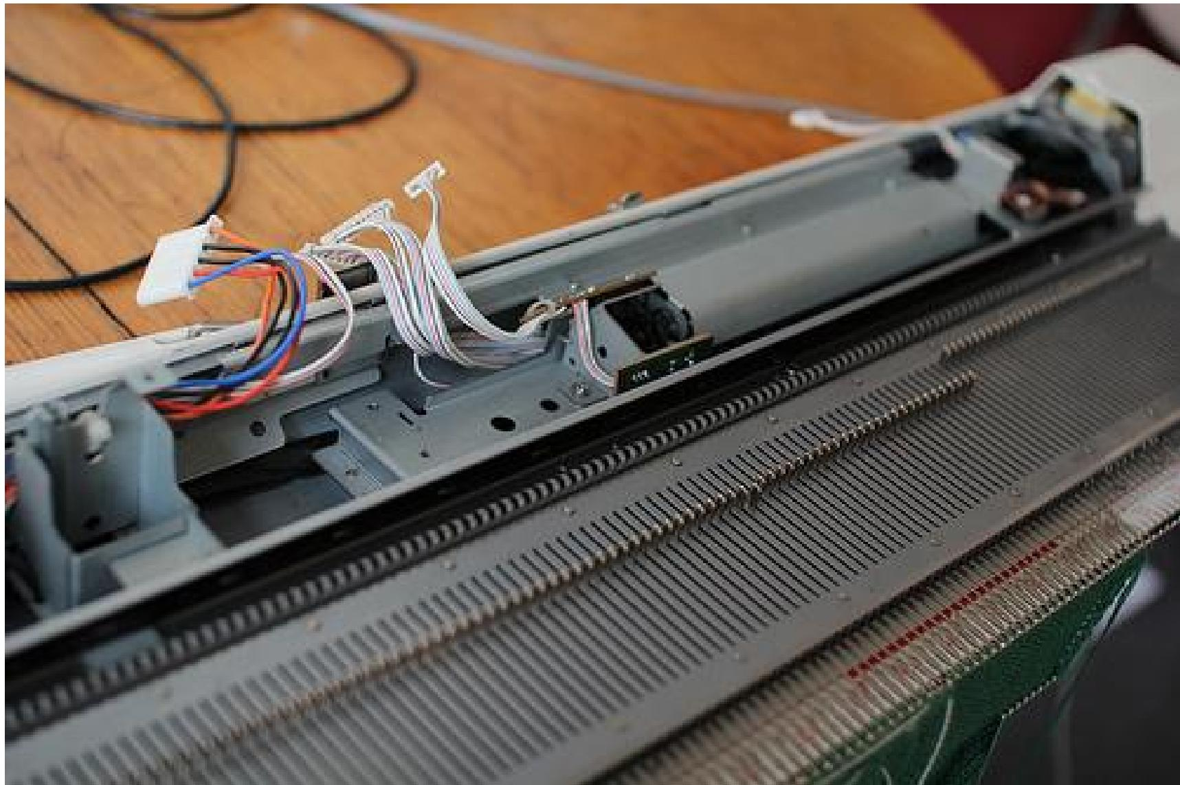
Step 3: plug all available wires coming from knitting machine into the Knitic (Arduino-based new brain)
